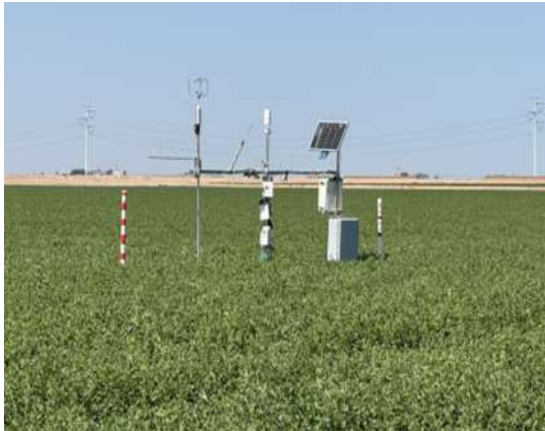
Figure 1. Eddy covariance tower and soil moisture monitoring system installed in a representative commercial alfalfa field for continuous monitoring of field-scale actual ET and root-zone soil water conditions under operational irrigation management.
